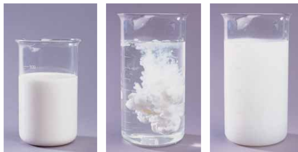
Mixing a suspension concentrate (SC) with water produces a suspension. The active substance is present as finely-distributed particles.
