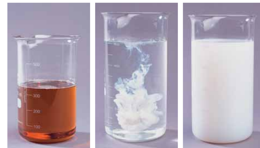
Diluting an emulsifiable concentrate (EC) in water produces an emulsion.
