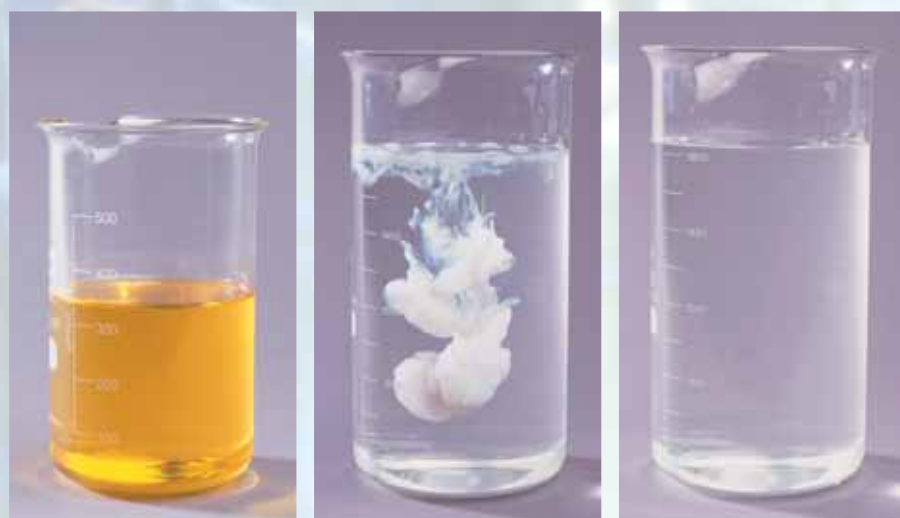
Dissolving a soluble concentrate (SL) in water results in a clear solution.
