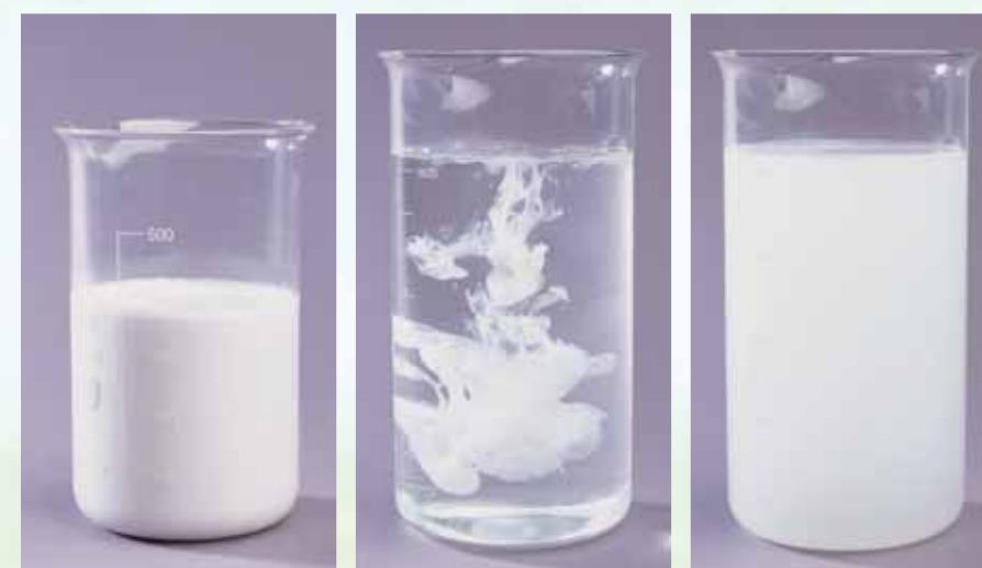
Mixing an oil dispersion (OD) with water results in a suspoemulsion.
